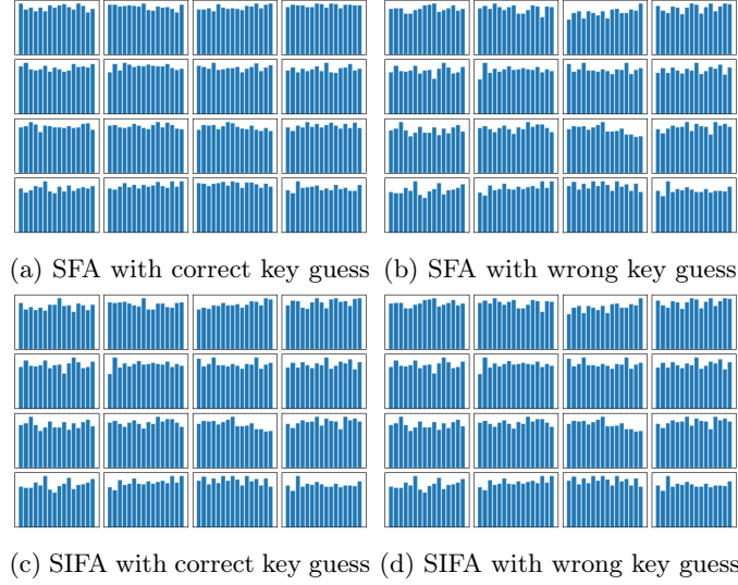
Fig. 8: Distribution of state nibbles after S-box in round 30 of the secure implementation after collecting 5000 ciphertexts. The distributions corresponding to SFA use all 5000 ciphertexts. The distributions corresponding to SIFA use 2477 correct ciphertexts out of 5000.
